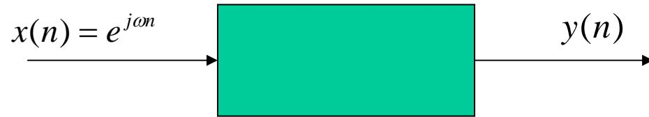
$$\begin{aligned} y(n) &= h(n) * x(n) = \sum_{m=0}^{\infty} h(m)e^{j\omega(n-m)} \\ &= [\sum_{m=0}^{\infty} h(m)e^{-j\omega m}]e^{j\omega n} = H(e^{j\omega})e^{j\omega n} \end{aligned}$$
