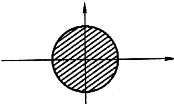
$$X(z) = \frac{z}{z - a}, z = 0 \text{零点}, z = a \text{极点}$$
